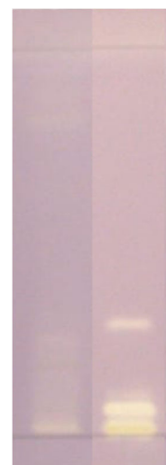
Fig 2. Chromatogram of EFC hexane (left lane) and EFC EtOAc (right lane) sprayed with DPPH• 5mM The mixture of n -hexane:CH 2 Cl 2 (1:9, v/v) was used as the mobile phase
